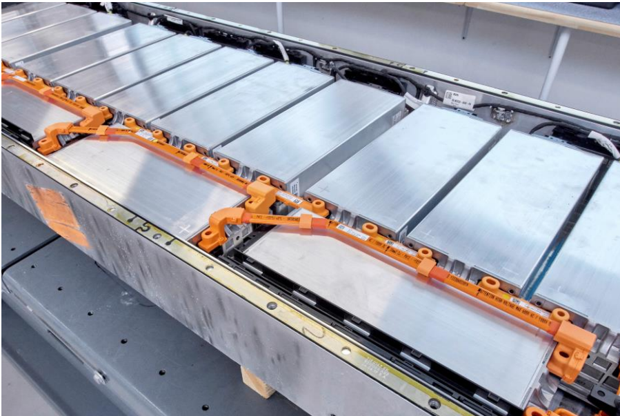
© MAN, Open battery from MAN in which the individual battery modules can be seen
