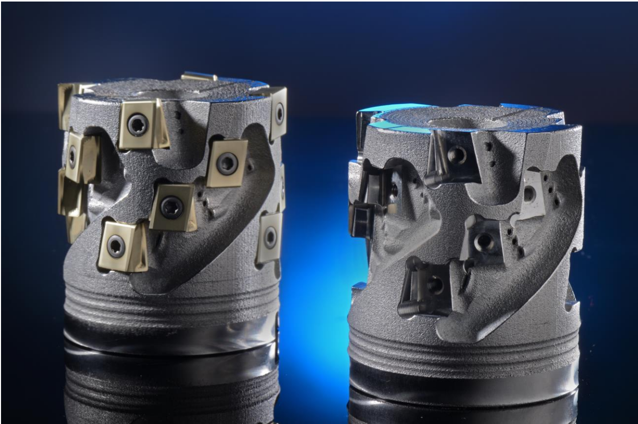
Multi-row demonstrator tool with low-loss and focused cutting fluid supply for use in aerospace structural components made of titanium alloys (©Fraunhofer ILT, Walter AG, Laboratory for Machine Tools and Production Engineering (WZL) of RWTH Aachen University)
