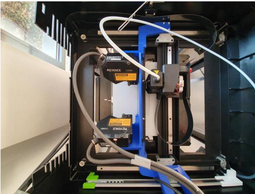
FDM printer with implemented laser light section sensors for in-process monitoring
