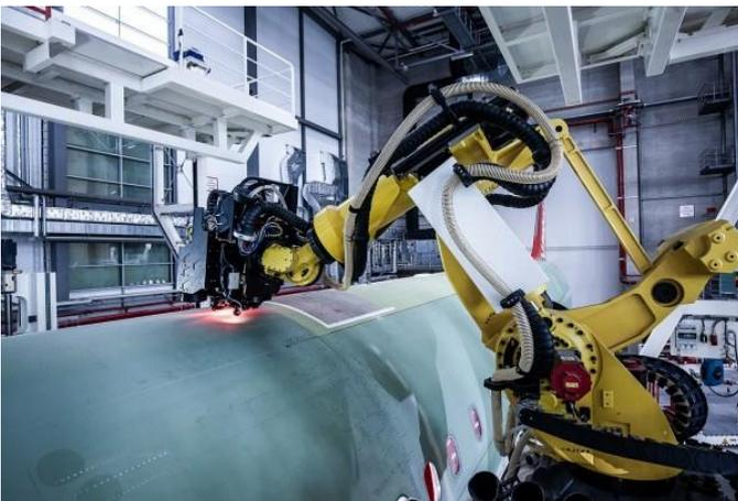
Robot-based final aircraft assembly: Highly accurate position data of the joining partners as well as of the robot end-effector are required for joining fuselage sections © Airbus
