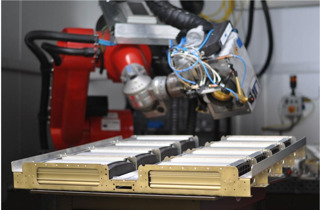
Jigless laser-welded low-cost battery pack housing made of high-strength aluminium (© WZL)
