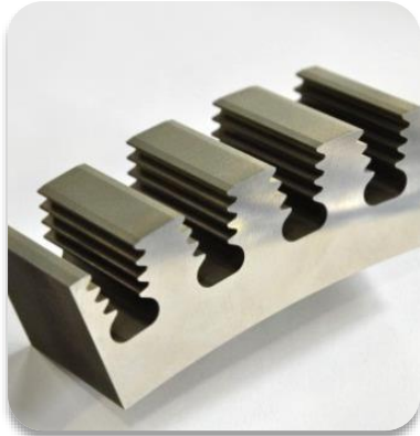
Drahtfunkenerosion von Profilnuten Wire EDM of fir tree slots
